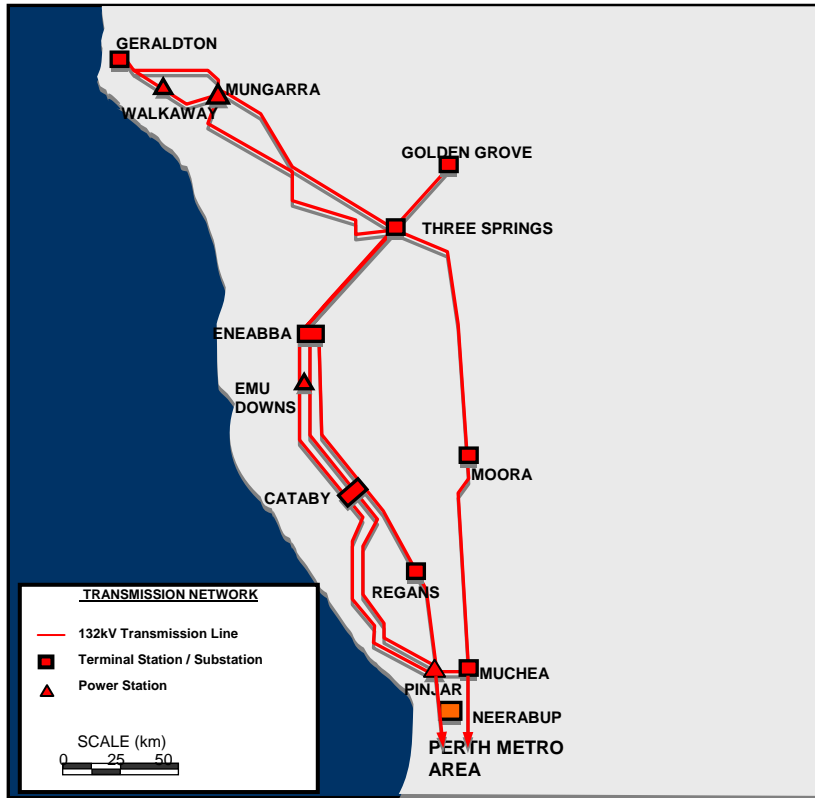
Figure 2 Mid West Region – existing network layout.
